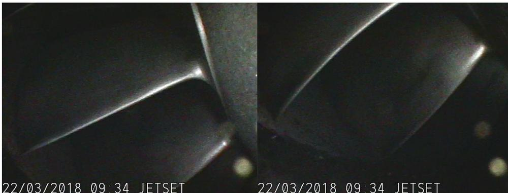
Coating loss on Intermediate case observed.
