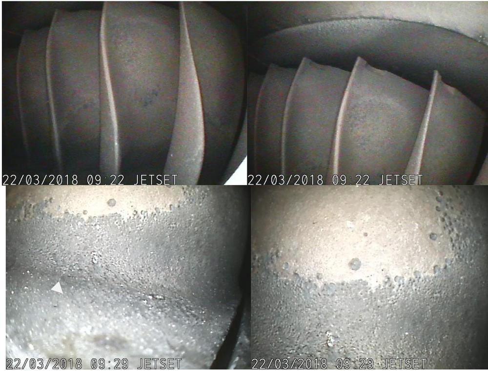
HT Vane Ring cracks noted on vanes and inner wall. IE duct No damage noted.
